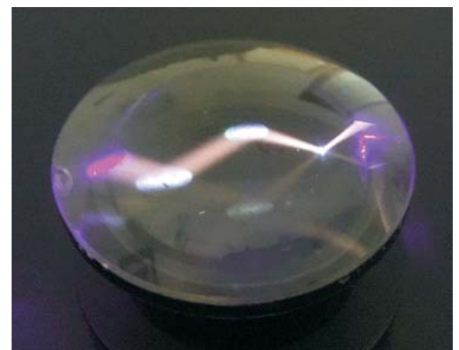
Fig.3. Origination of stray light in optical lens. Light of 405 nm laser pointer is invisible in clean air, but visualized at the surface and in the bulk of the lens due to scatter, reflections, and auto-fluorescence.
