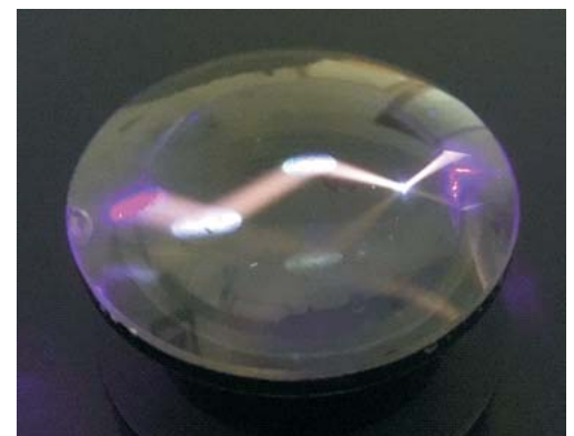
Fig.3. Origination of stray light in optical lens. Light of 405 nm laser is invisible in clean air, but visualized at the surface and in the bulk of the lens due to scatter, reflections, and auto-fluorescence.
