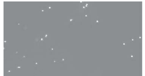
Fig. 9. Objective-based TIRF,100X, NA 1.46 oil-imm. objective. 1-um fluorescent beads.
