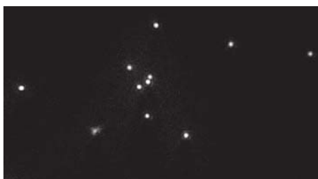
Fig.7. Prism-based TIRF,100X, NA 1.25 oil-imm. objective. 1-micron fluorescent beads.
